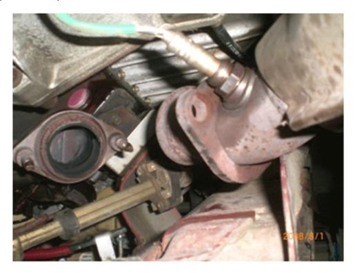
10. Now, very carefully, pull the headers out. I found it was easier to remove one header through the bottom on the left side, and the other header through the top on the right side.
